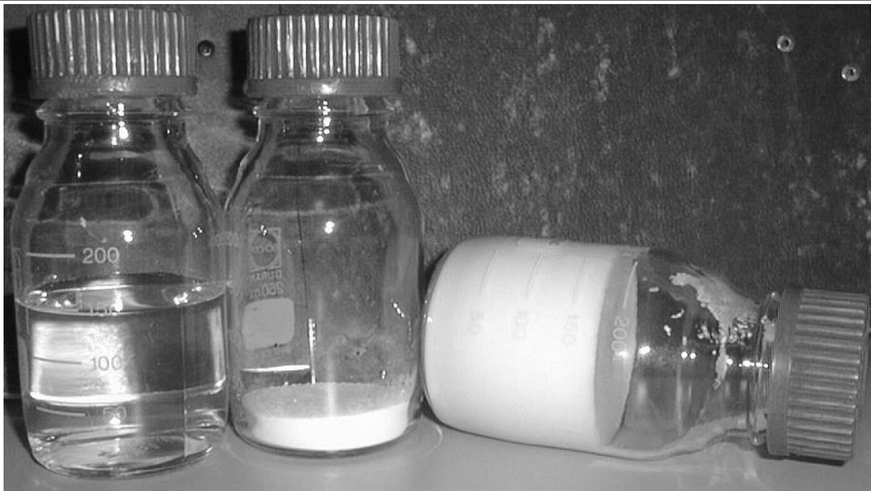
100g methanol ( \approx 150\text{ml} , left); 10g NaKGA monohydrate (centre), after suspending the hydrate in methanol (right)
